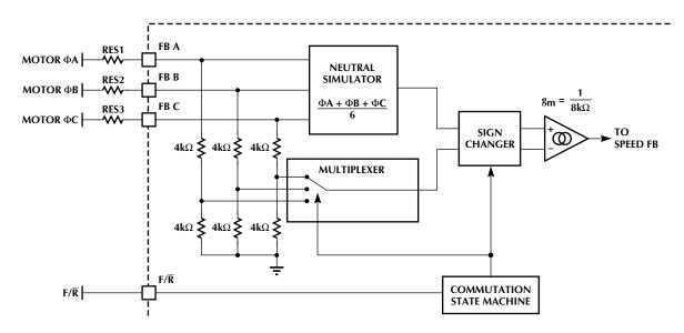
Figure 6. Back EMF Sampler Detailed Block Diagram
