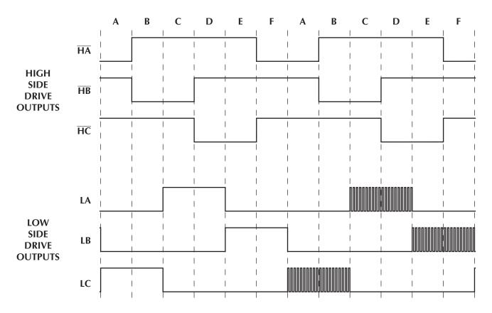
Figure 4. Output Commutation Sequence Timing Diagram
