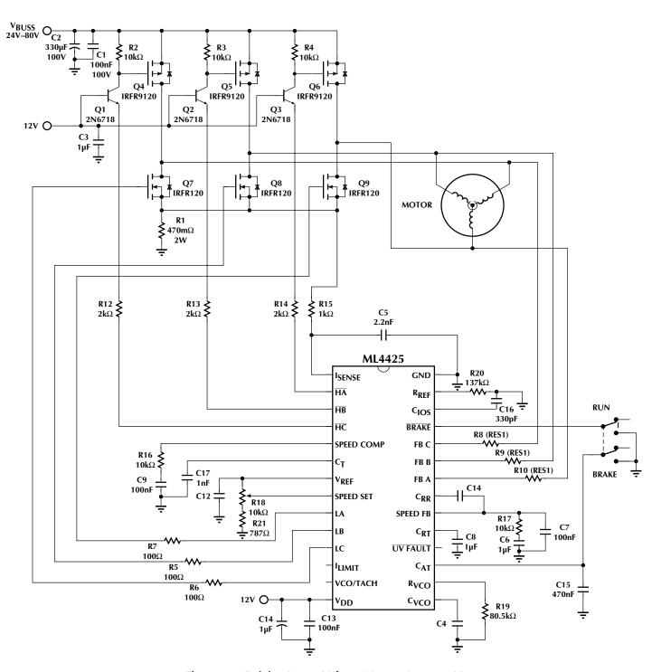
Figure 11. Driving Lower Voltage Motors (12 to 80V)
