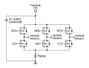
Figure 1. Using R<sub>SENSE</sub> in a 3-Phase 12V Power Stage
