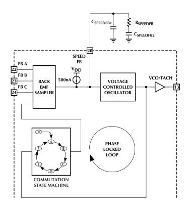
Figure 7. Back EMF Commutation Phase Locked Loop
