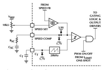
Figure 9. Speed Control Loop Component Connections
