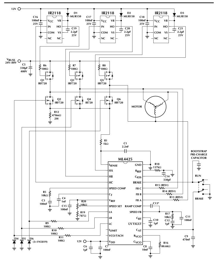
Figure 12. ML4425 High Voltage Motor Drive Application Circuit
