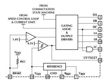
Figure 10. Cross Conduction, Brake, and UVLO Circuits
