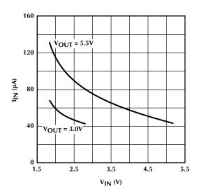
Figure 6. No Load Input Current vs. VIN
