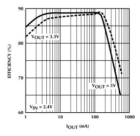
Figure 5. Efficiency vs. I<sub>OUT</sub> Using the Circuit of Figure 8
