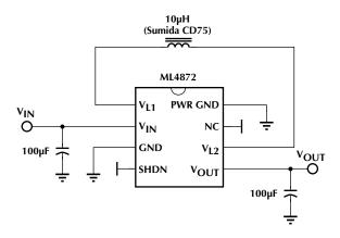
Figure 8. Typical Application Circuit
