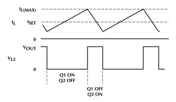
Figure 3. Inductor Current and Voltage Waveforms
