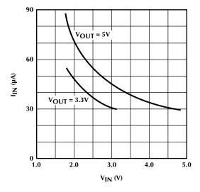
Figure 6. No Load Input Current vs. V<sub>IN</sub>
