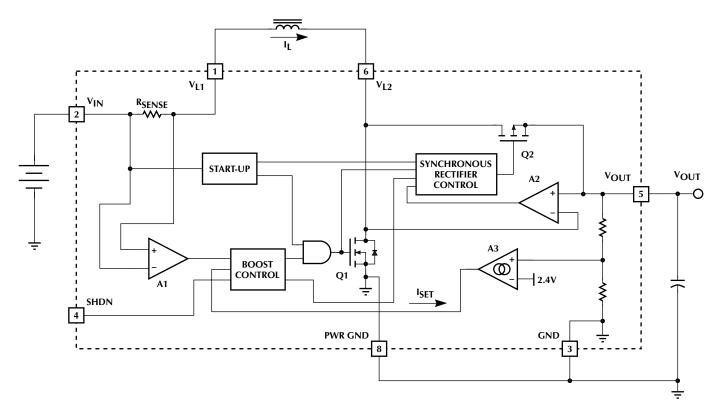
Figure 2. PFM Regulator Block Diagram
