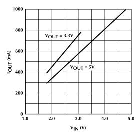
Figure 4. I<sub>OUT</sub> vs. VIN Using the Circuit of Figure 8
