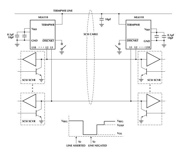
Figure 2. Application Diagram Showing Typical SCSI Bus Configuration with the ML6518
