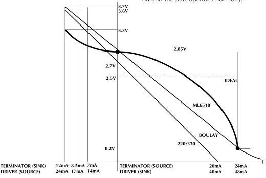
Figure 1. V-1 Characteristics of Various SCSI Termination Schemes
