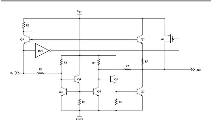
Figure 5. One buffer cell of the ML65T541
