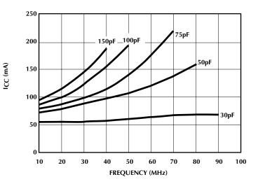
Figure 4. I<sub>CC</sub> Versus Frequency for Various Load Capacitances, Four Outputs Switching.
