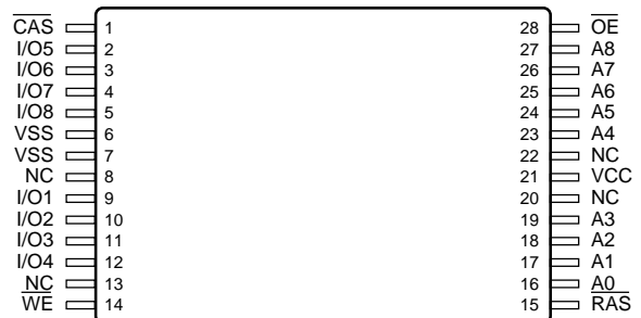
28 Lead TSOP-I PIN CONFIGURATION Top View
