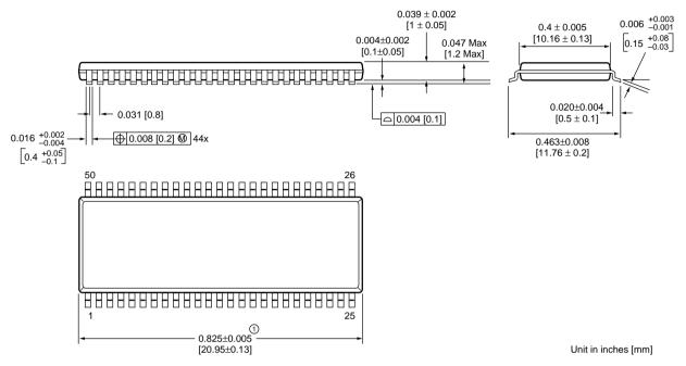
1 Does not include plastic or metal protrusion of 0.010 [0.25] max. per side
