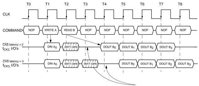
Input data must be removed from the I/O's at least one clock cycle before the Read dataAPpears on the outputs to avoid data contention.
