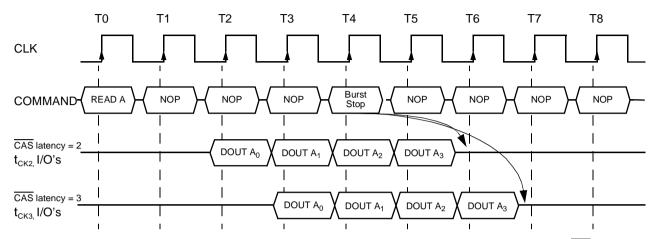
The burst ends after a delay equal to the  $\overline{\text{CAS}}$  latency.
