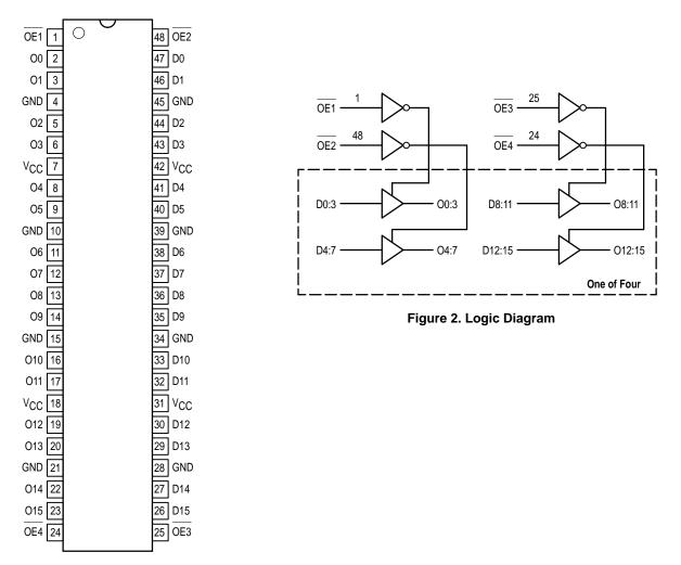
Figure 1. 48–Lead Pinout (Top View)
