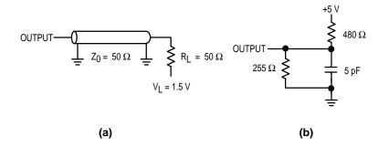
Figure 1. AC Test Loads
