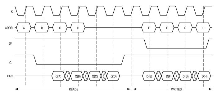
Figure 2. Configured as Non-Burst Pipelined Synchronous SRAM
