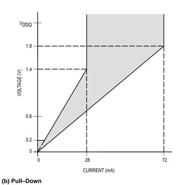
Figure 7. Typical Output Buffer Characteristics – PBGA Only
