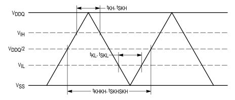
Figure 6. AC Timing Diagram Clock Reference
