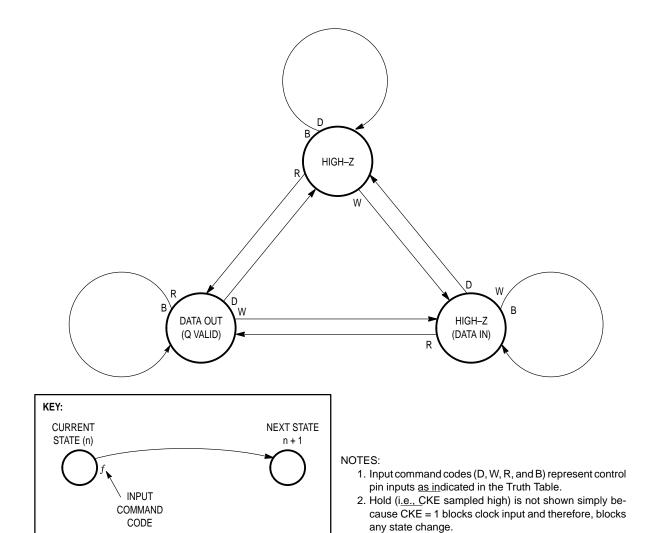
Figure 3. Data I/O State Diagram
