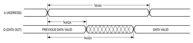
NOTE: Device is continuously selected ( $\overline{E}$  = V<sub>IL</sub>,  $\overline{G}$  = V<sub>IL</sub>).
