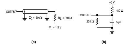
Figure 1. AC Test Loads
