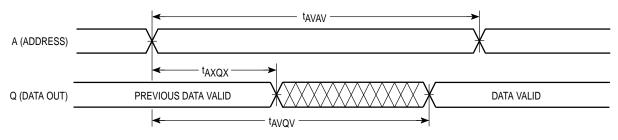
NOTE: Device is continuously selected ( $\overline{E} = V_{IL}, \overline{G} = V_{IL}$ ).
