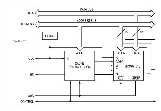
256K Byte Burstable, Secondary Cache Using Four MCM67J518FN7s with a 75 MHz (Bus Speed) Pentium
