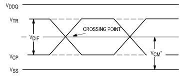
$^*$ V<sub>CM</sub>, the Common Mode Input Voltage, equals  $V_{TR} - ((V_{TR} - V_{CP})/2)$ .
