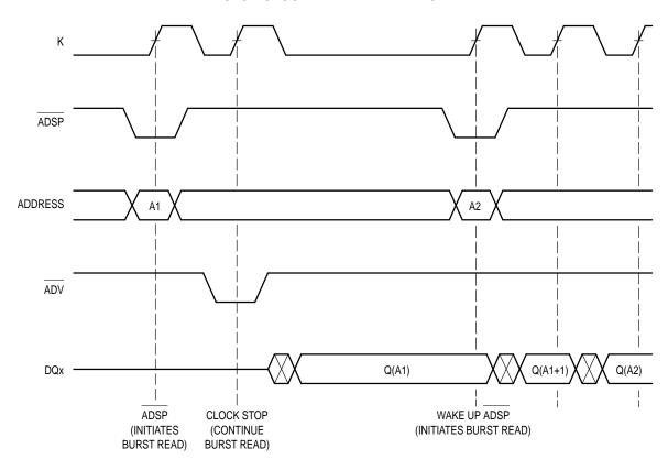
NOTE: For lowest possible power consumption during stop clock, the addresses should be driven to a low state ( $V_{IL}$ ). Best results are obtained if  $V_{IL} < 0.2 \text{ V}$ .
