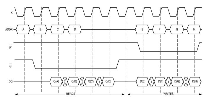
Figure 5. Configured as Non-Burst Synchronous SRAM
