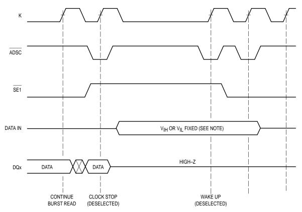
NOTE: While the clock is stopped, DATA IN must be fixed in a high (V<sub>IH</sub>) or low (V<sub>IL</sub>) state to reduce the DC current of the input buffers. For lowest power operation, all data and address lines should be held in a low (V<sub>IL</sub>) state and control lines held in an inactive state.
