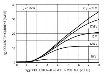
Figure 2. Output Characteristics,  $T_J = 125^{\circ}C$
