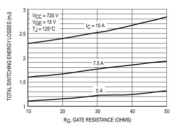
Figure 7. Total Switching Losses versus Gate Resistance
