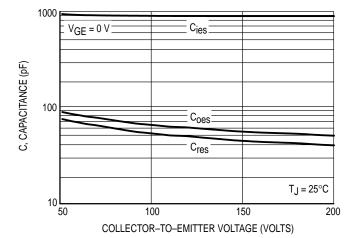
Figure 5b. High Voltage Capacitance Variation
