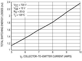
Figure 9. Total Switching Losses versus Collector-to-Emitter Current
