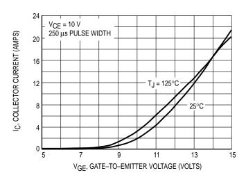
Figure 3. Transfer Characteristics
