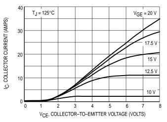
Figure 2. Output Characteristics, T<sub>J</sub> = 125°C
