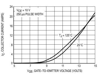
**Figure 3. Transfer Characteristics**
