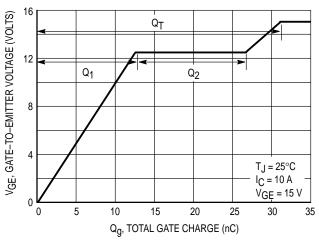
Figure 6. Gate-to-Emitter Voltage versus Total Charge
