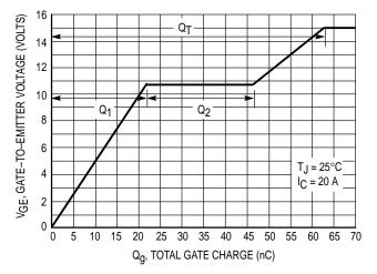
Figure 6. Gate-to-Emitter Voltage versus
