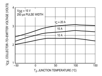
Figure 4. Collector-to-Emitter Saturation Voltage versus Junction Temperature
