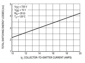
Figure 9. Turn-Off Losses versus Collector-to-Emitter Current
