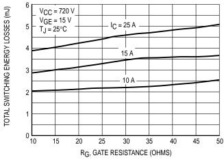
Figure 7. Total Switching Losses versus
