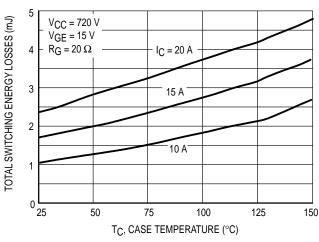
Figure 8. Total Switching Losses versus
