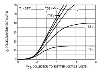
Figure 1. Output Characteristics, T<sub>J</sub> = 25°C
