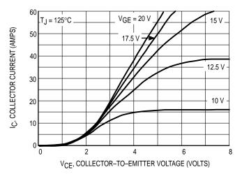
Figure 2. Output Characteristics, T<sub>J</sub> = 125°C
