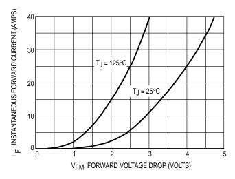
Figure 10. Maximum Forward Drop versus Instantaneous Forward Current
