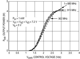
Figure 4. Output Power versus Control Voltage
