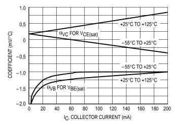
Figure 18. Temperature Coefficients
