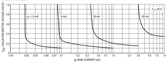
Figure 16. Collector Saturation Region
