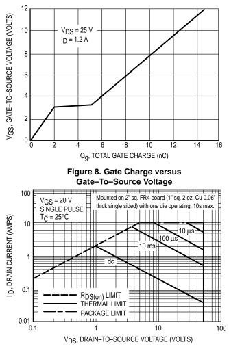
Figure 9. Maximum Rated Forward Biased Safe Operating Area
