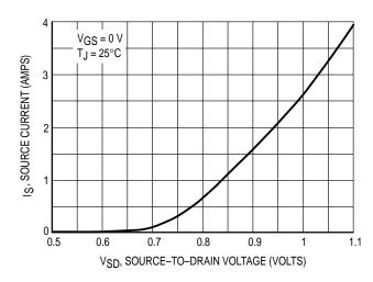
Figure 10. Diode Forward Voltage versus Current
