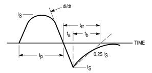
Figure 15. Diode Reverse Recovery Waveform
