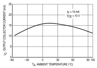
Figure 4. Output Current versus Ambient Temperature
