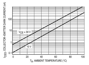
Figure 5. Dark Current versus Ambient Temperature
