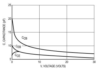
Figure 6. Capacitances versus Voltage
