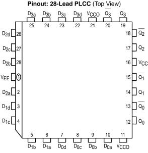
$^{\ast}$  All V<sub>CC</sub> and V<sub>CCO</sub> pins are tied together on the die.
