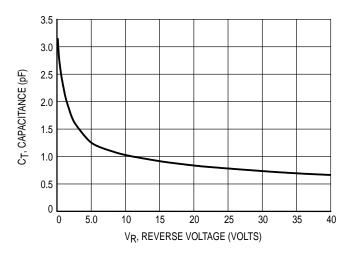
Figure 3. Typical Capacitance
