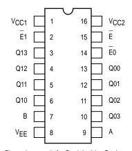
Pin assignment is for Dual–in–Line Package. For PLCC pin assignment, see the Pin Conversion Tables on page 6–36 of the Motorola MECL Data Book (DL122/D).
