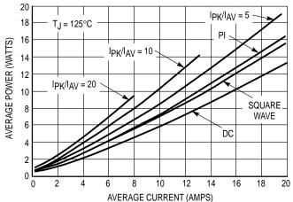
Figure 3. Typical Current Derating, Case, Per Leg
