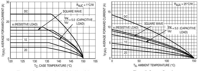
Figure 6. Current Derating, Infinite Heatsink
