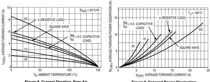
Figure 8. Current Derating, Free Air
