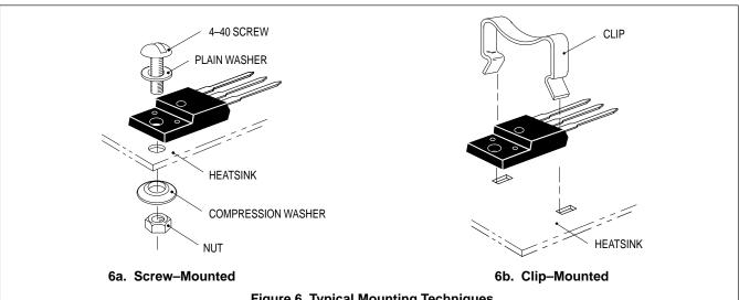
**Figure 6. Typical Mounting Techniques**
