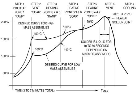
Figure 12. Typical Solder Heating Profile
