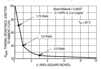
Figure 10. Thermal Resistance versus Drain Pad Area for the D<sup>3</sup>PAK Package (Typical)
