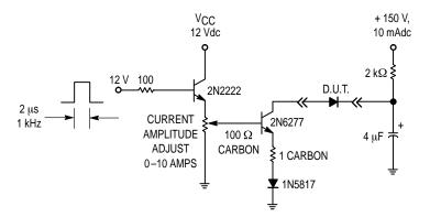
Figure 9. Test Circuit for Repetitive Reverse Current
