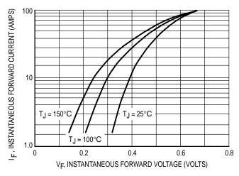
Figure 1. Typical Forward Voltage
