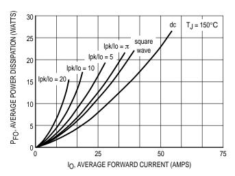
Figure 6. Forward Power Dissipation (Per Leg)
