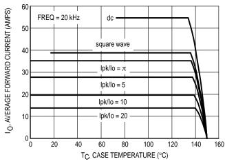
Figure 5. Current Derating (Per Leg)
