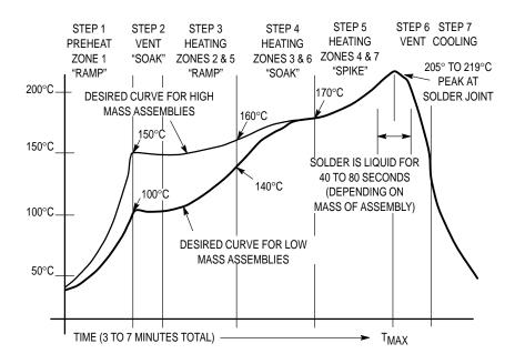
Figure 4. Typical Solder Heating Profile
