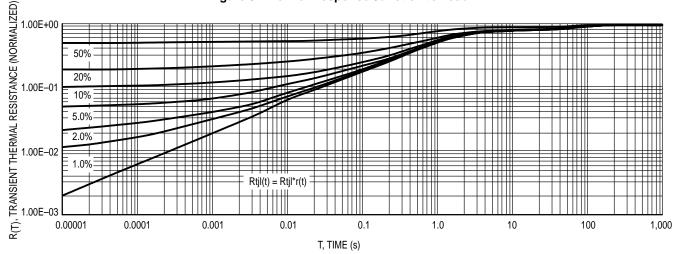
Figure 10. Thermal Response Junction to Ambient
