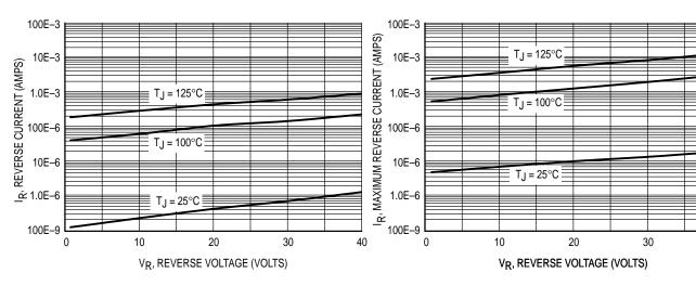
**Figure 3. Typical Reverse Current**
