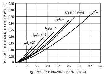
Figure 6. Forward Power Dissipation
