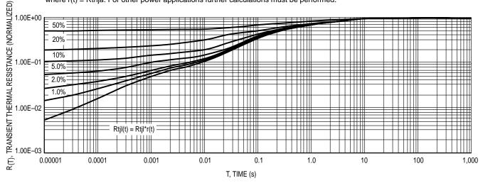
Figure 9. Thermal Response Junction to Lead
