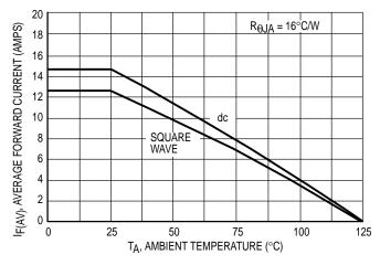
Figure 5. Current Derating Ambient, Per Leg
