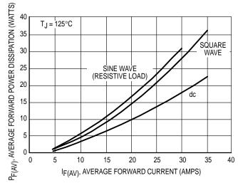
Figure 3. Forward Power Dissipation, Per Leg
