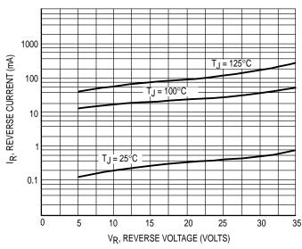
Figure 2. Typical Reverse Current, Per Leg
