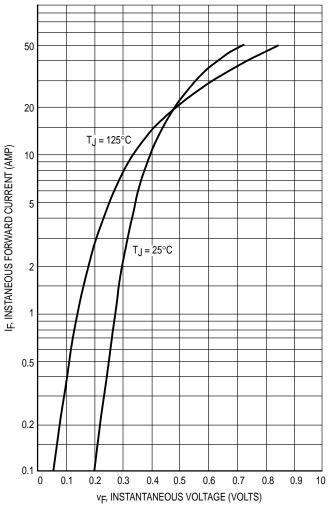
Figure 1. Typical Forward Voltage, Per Leg
