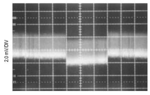
V<sub>ref</sub> LOAD REGULATION 1.0 mA to 10 mA (2.0 ms/DIV)
