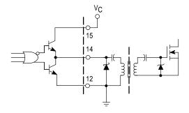
The totem pole output can easily drive pulse transformers. A Schottky diode is recommended when driving inductive loads at high frequencies. The diode can reduce the driver's power dissipation due to excessive ringing, by preventing the output pin from being driven below ground.
