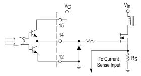
A series gate resistor may be needed to dampen high frequency parasitic oscillation caused by the MOSFET's input capacitance and any series wiring inductance in the gate–source circuit. The series resistor will also decrease the MOSFET switching speed. A Schottky diode can reduce the driver's power dissipation due to excessive ringing, by preventing the output pin from being driven below ground. The Schottky diode also prevents substrate injection when the output pin is driven below ground.
