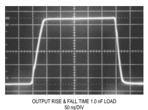
Figure 16. Drive Output Rise and Fall Time
