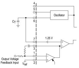
In voltage mode operation, the control range on the output of the Error Amplifier from 0% to 90% duty cycle is from 2.25 V to 4.05 V.
