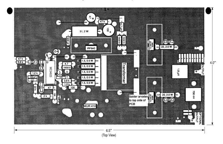
**Figure 36. PC Board Without Components**
