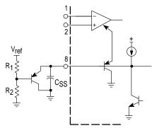
In voltage mode operation, the maximum duty cycle can be clamped. By the addition of a PNP transistor to buffer the clamp voltage, the Soft–Start current is not affected by  $\mathsf{R}_1$ .
