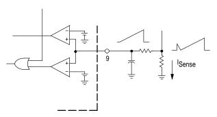
The addition of an RC filter will eliminate instability caused by the leading edge spike on the current waveform. This sense signal can also be used at the ramp input pin for current mode control. For ramp compensation it is necessary to know the gain of the current feedback loop. If a transformer is used, the gain can be calculated by:
