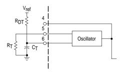
Additional dead time can be added by the addition of a dead time resistor from  $V_{\mbox{\scriptsize ref}}$  to  $C_{\mbox{\scriptsize T}\!.}$  See text on Oscillator section for more information.
