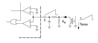
The addition of an RC filter will eliminate instability caused by the leading edge spike on the current waveform. This sense signal can also be used at the ramp input pin for current mode control. For ramp compensation it is necessary to know the gain of the current feedback loop. The gain can be calculated by:
