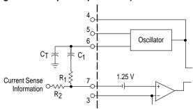
This method of slope compensation is easy to implement, however, it is noise sensitive. Capacitor  $\mathsf{C}_1$  provides AC coupling. The oscillator signal is added to the current signal by a voltage divider consisting of resistors  $\mathsf{R}_1$  and  $\mathsf{R}_2$ .
