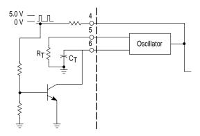
The sync pulse fed into the clock pin must be at least  $3.9 \, \text{V}$ .  $R_T$  and  $C_T$  need to be set 10% slower than the sync frequency. This circuit is also used in Voltage Mode operation for master/slave operation. The clock signal would be coming from the master which is set at the desired operating frequency, while the slave is set 10% slower.
