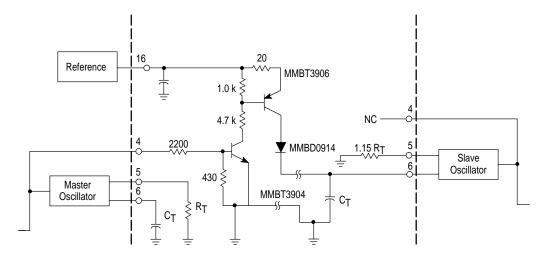
Figure 30. Buffered Maximum Clamp Level
