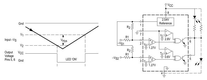
The above figure shows the MC34161 configured as a dual negative overvoltage detector. As the input voltage increases from ground, the LED will turn 'ON' when -V<sub>S1</sub> or -V<sub>S2</sub> exceeds V<sub>2</sub>. With the dashed line output connection, the circuit becomes a dual negative undervoltage detector. As the input voltage decreases from the peak towards ground, the LED will turn 'ON' when  $-V_{S1}$  or  $-V_{S2}$  falls below  $V_1$ .
