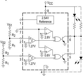
The above figure shows the MC34161 configured as a dual positive undervoltage detector. As the input voltage decreases towards ground, the LED will turn 'ON' when  $V_{S1}$  or  $V_{S2}$  falls below  $V_1$ . With the dashed line output connection, the circuit becomes a dual positive overvoltage detector. As the input voltage increases from ground, the LED will turn 'ON' when  $V_{S1}$  or  $V_{S2}$  exceeds  $V_2$ .
