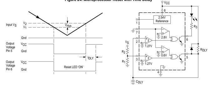
Figure 24. Microprocessor Reset with Time Delay
