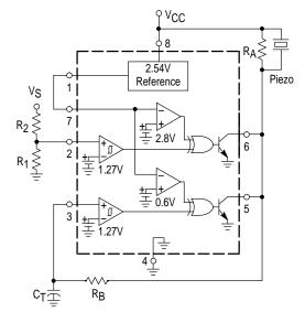
The above figure shows the MC34161 configured as an overvoltage detector with an audio alarm. Channel 1 monitors input voltage  $V_S$  while channel 2 is connected as a simple RC oscillator. As the input voltage increases from ground, the output of channel 1 allows the oscillator to turn 'ON' when  $V_S$  exceeds  $V_2$ .
