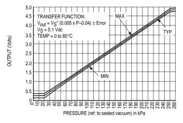
Figure 4. Output versus Absolute Pressure
