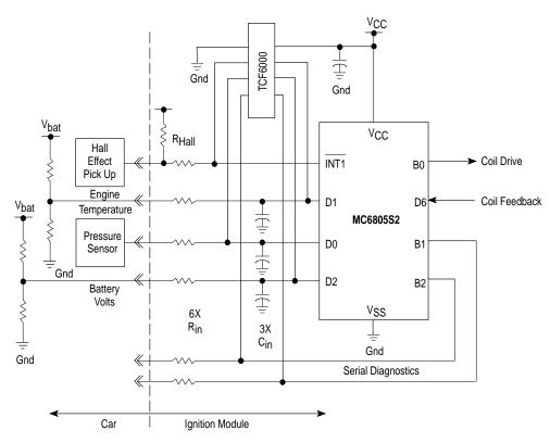
The use of  $C_{in}$  is not mandatory, and is not recommended where the lines to be protected are used for output or for both input and output. For digital input lines, the use of a small capacitor in the range of 50 pF to 220 pF is recommended as this will reduce the rate of rise of voltage seen by the TCF6000 and hence the possibility of overshoot.
