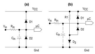
Figure 3 shows the clamping characteristics which are common to each of the six cells in the Peripheral Clamping Array.
