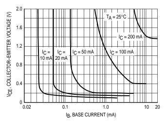
Figure 3. Collector Saturation Region
