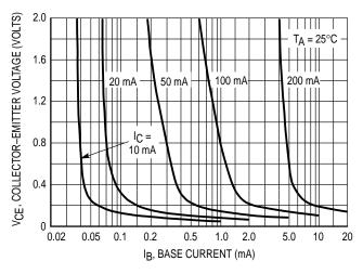
Figure 9. Collector Saturation Region
