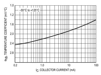
Figure 4. Base-Emitter Temperature Coefficient
