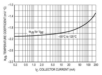
Figure 10. Base-Emitter Temperature Coefficient
