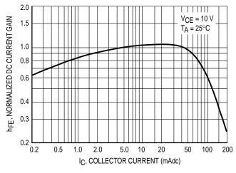
Figure 1. Normalized DC Current Gain
