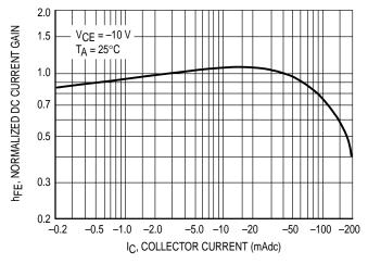
Figure 1. Normalized DC Current Gain
