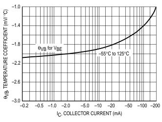
Figure 10. Base-Emitter Temperature Coefficient
