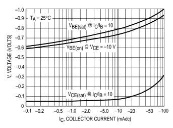
Figure 2. "Saturation" and "On" Voltages
