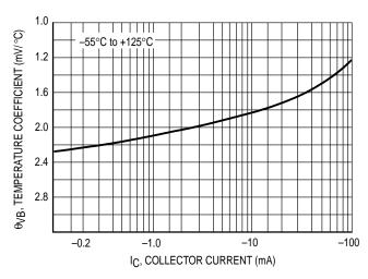
Figure 4. Base-Emitter Temperature Coefficient
