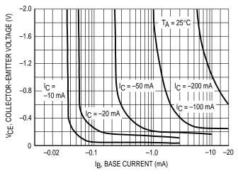
Figure 3. Collector Saturation Region
