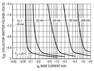
Figure 9. Collector Saturation Region
