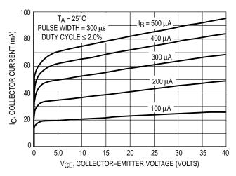
**Figure 9. Collector Characteristics**
