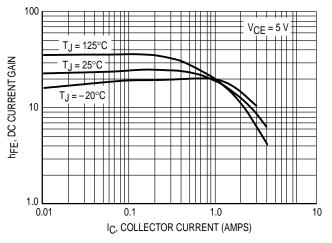
Figure 2. DC Current Gain at 5 Volts
