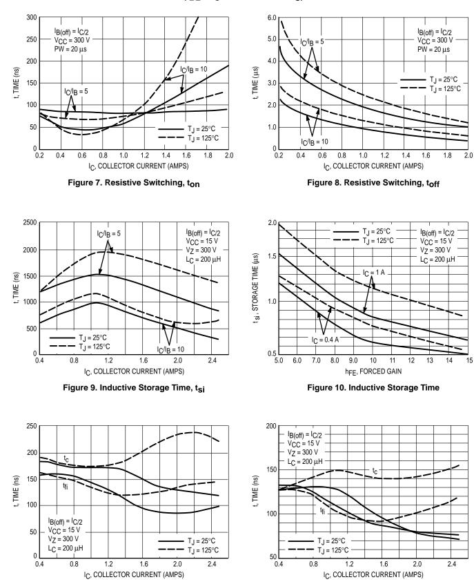
TYPICAL SWITCHING CHARACTERISTICS (IB2 = IC/2 for all switching)
