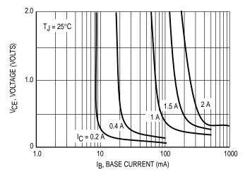
Figure 3. Collector Saturation Region
