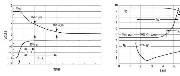
Figure 18. Dynamic Saturation Voltage Measurements
