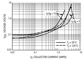
Figure 4. Collector–Emitter Saturation Voltage
