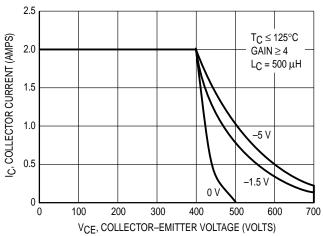
Figure 16. Reverse Bias Switching Safe Operating Area
