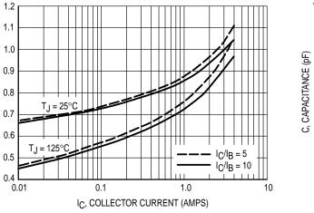
Figure 5. Base–Emitter Saturation Region
