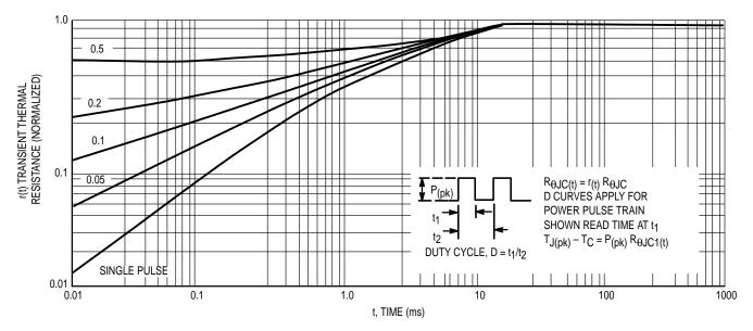
Figure 21. Typical Thermal Response (Z $_{\theta JC}(t)$ ) for BUL44F
