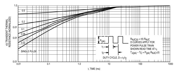
Figure 20. Typical Thermal Response ( $Z_{\theta JC}(t)$ ) for BUL44
