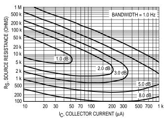
Figure 5. Narrow Band, 100 Hz
