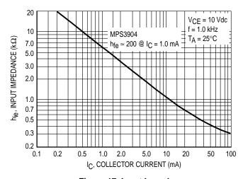
Figure 17. Input Impedance
