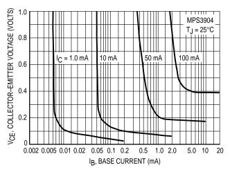
Figure 9. Collector Saturation Region
