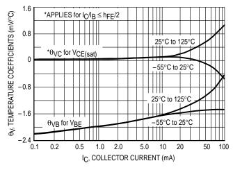
Figure 12. Temperature Coefficients
