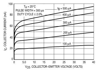
Figure 10. Collector Characteristics
