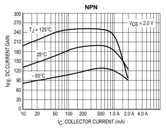
Figure 1. MPS650, MPS651 Typical DC Current Gain
