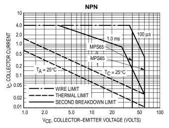
Figure 7. MPS650, MPS651 SOA, Safe Operating Area
