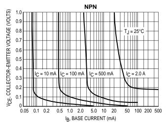
Figure 5. MPS650, MPS651 Collector Saturation Region
