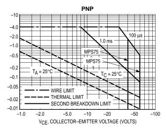
Figure 8. MPS750, MPS751 SOA, Safe Operating Area
