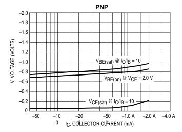
Figure 4. MPS750, MPS751 On Voltages
