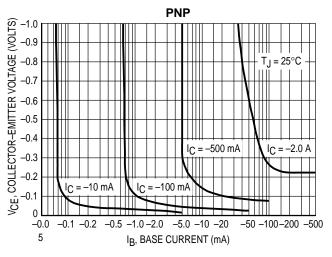
Figure 6. MPS750, MPS751 Collector Saturation Region
