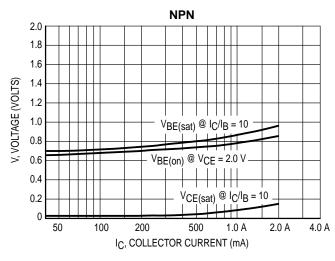
Figure 3. MPS650, MPS651 On Voltages
