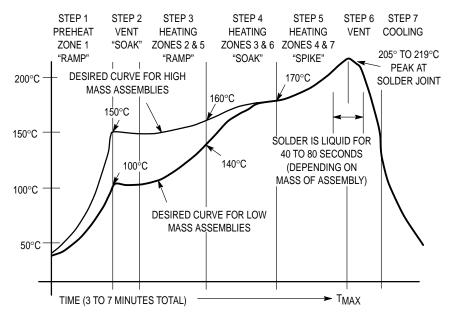
Figure 1. Typical Solder Heating Profile
