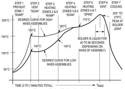
Figure 8. Typical Solder Heating Profile
