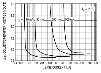
Figure 5. Collector Saturation Region
