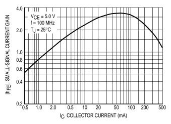
**Figure 2. High Frequency Current Gain**
