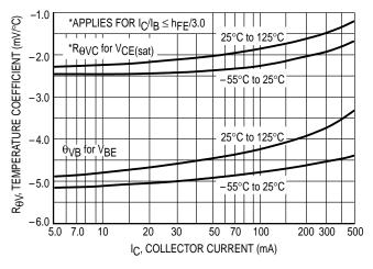
Figure 6. Temperature Coefficients
