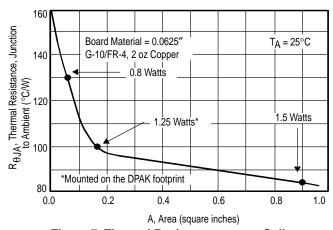
Figure 7. Thermal Resistance versus Collector Pad Area for the SOT-223 Package (Typical)
