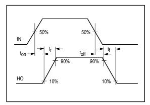
Figure 2. Switching Time Waveform Definitions
