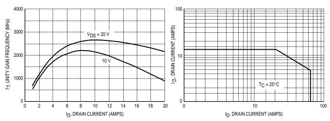
Figure 3. Common Source Unity Current Gain Frequency versus Drain Current
