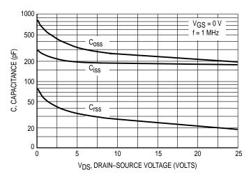
Figure 7. Capacitance versus Drain-Source Voltage
