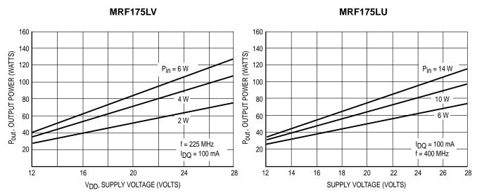
Figure 8. Output Power versus Supply Voltage
