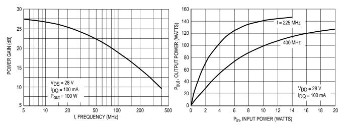
Figure 10. Power Gain versus Frequency
