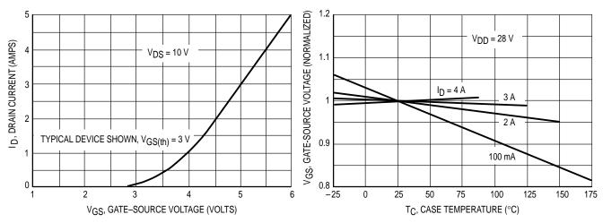
Figure 5. Drain Current versus Gate Voltage (Transfer Characteristics)
